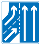
Additional traffic joining from left ahead. Traffic on main carriageway has priority over joining traffic from right-hand lane of slip road
