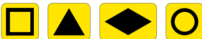
Symbols showing emergency diversion route for motorway and other main road traffic
