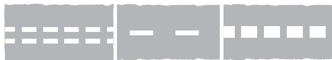
Give way to traffic on major road (can also be used at mini roundabouts)
